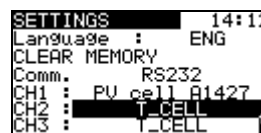
Figure 3-6: Use of temperature sensor selection
