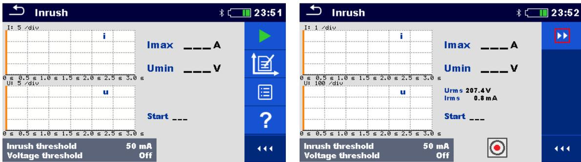
Figure E.10: Inrush current menu – setup on the left, waiting for trigger on the right
